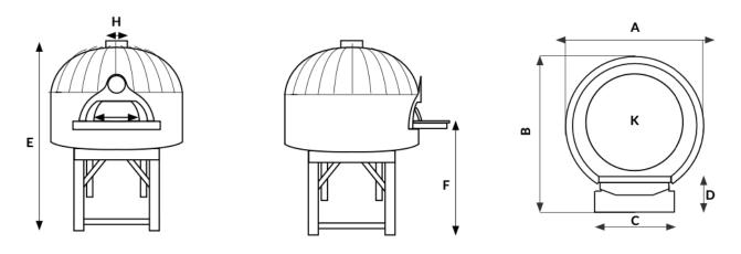
A Oven Width | B Oven Depth | C Frontal Width | D Frontal Depth | E Oven Height
